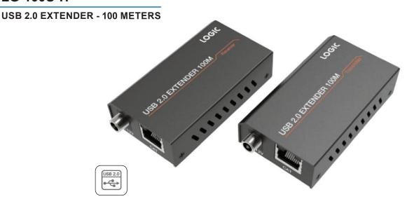
The USB2.0 extender can easily send the USB signals via CAT 5e/6 cables up to 100 meters /328 ft. at the transmission rate of 200 Mbps. Without any configuration or software driver. In a transmitter, the USB-B port has connected to a PC. In the receiver, you can connect a device with a USB port at the two USB ports such as a U disk or printer.
