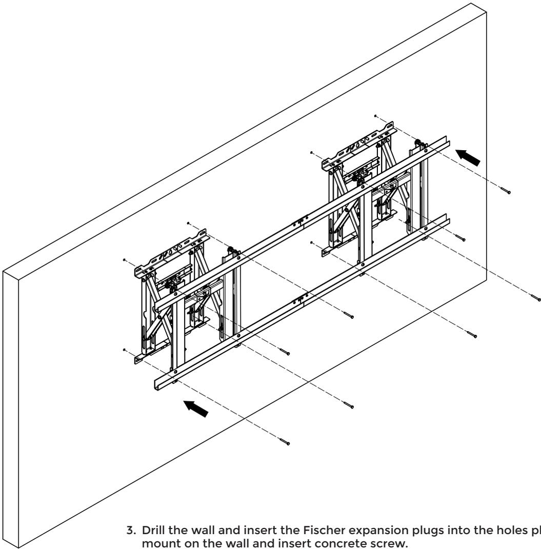
3. Drill the wall and insert the Fischer expansion plugs into the holes place the mount on the wall and insert concrete screw.
