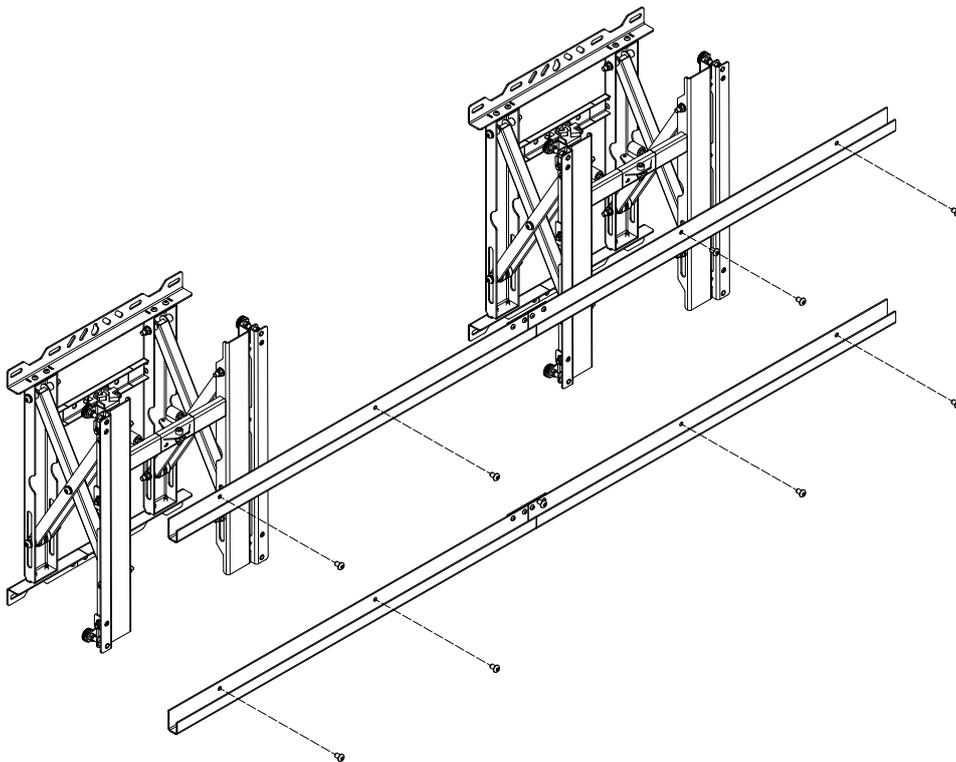
Fix the whole connecting bar to the wall mount bracket as show in image.
