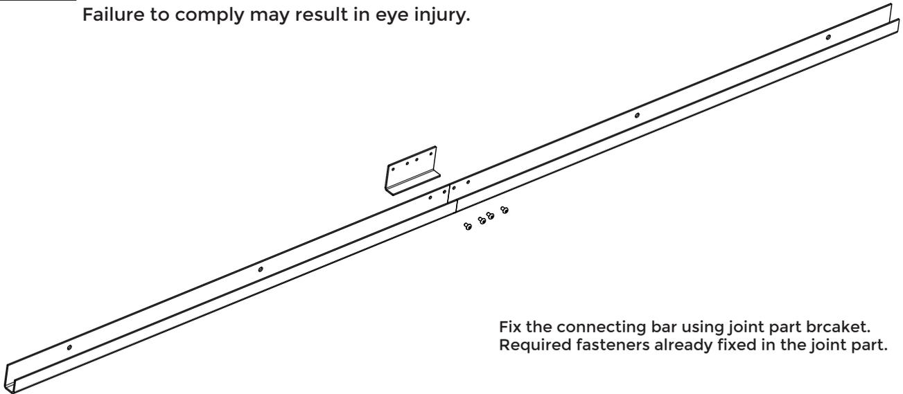
Fix the connecting bar using joint part bracket.
