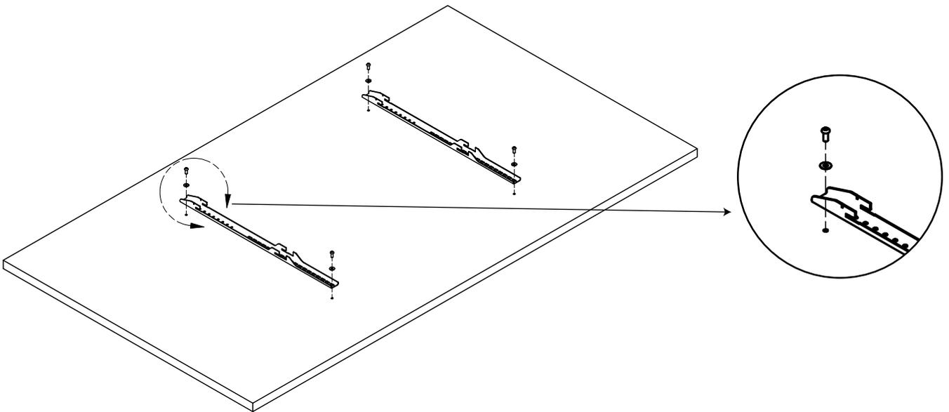
4. Place the interface bracket on the TV/ display and insert the washer and screw.
