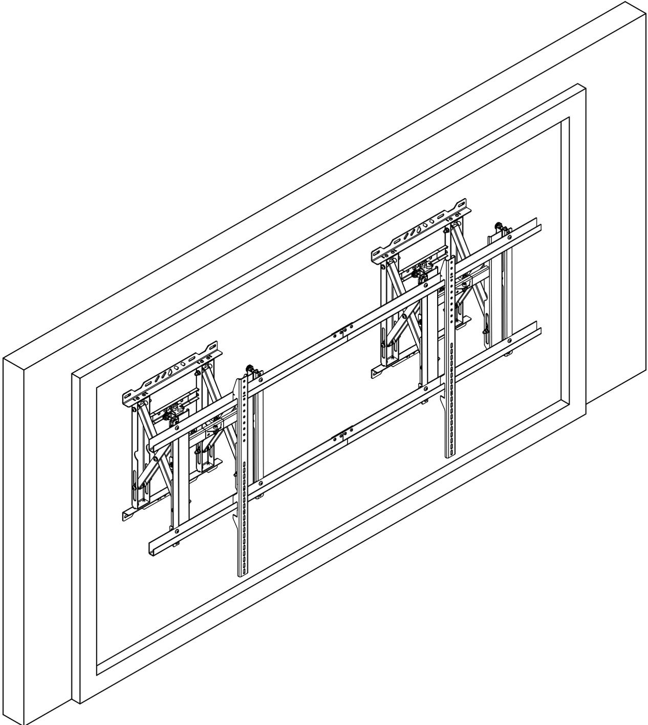
NOTE - Display cannot be unlocked at one push in middle. Since the display size is large.
