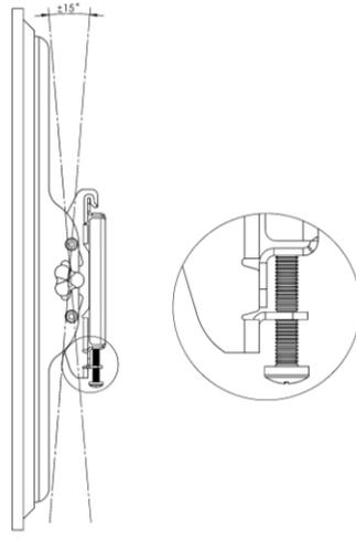
5. Adjust the angle and lock the mount
