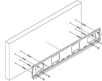
1. Place the wall unit on the wall and make marks on the wall.
