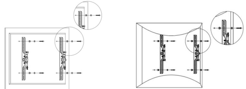
2. Place the interface bracket on the TV/ display and insert the washer and screw (Refer the checklist for the suitable screw and washer)
