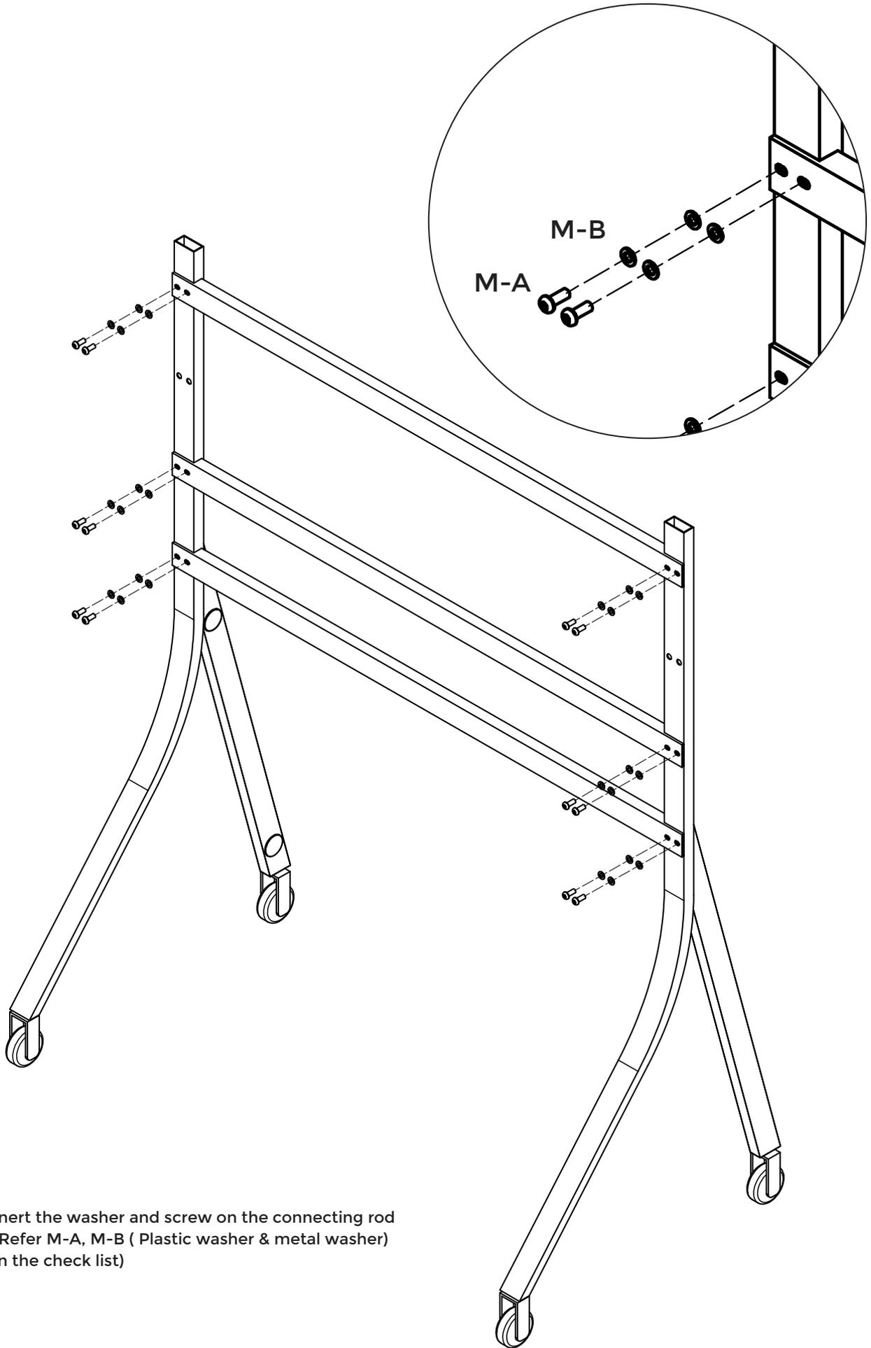
3. Inert the washer and screw on the connecting rod
