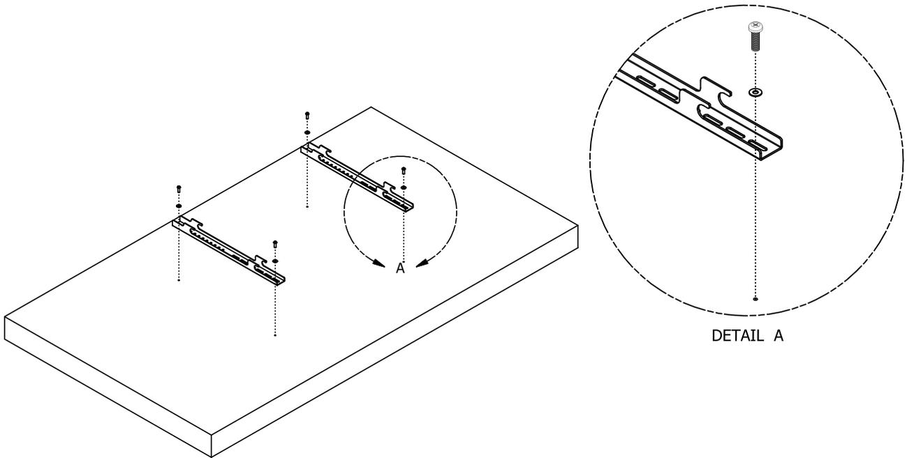
6. Place the interface bracket on the TV/ display and insert washer and screw (Refer the checklist for the suitable screw (M-C, M-E, M-G) and washer ( M-D, M-F, M-H) for the display/TV)
