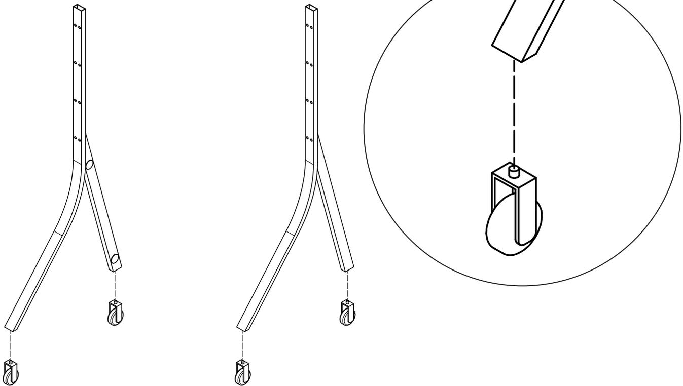
1. Place the castors to bottom side of the base left and right rail and tighten the castors
