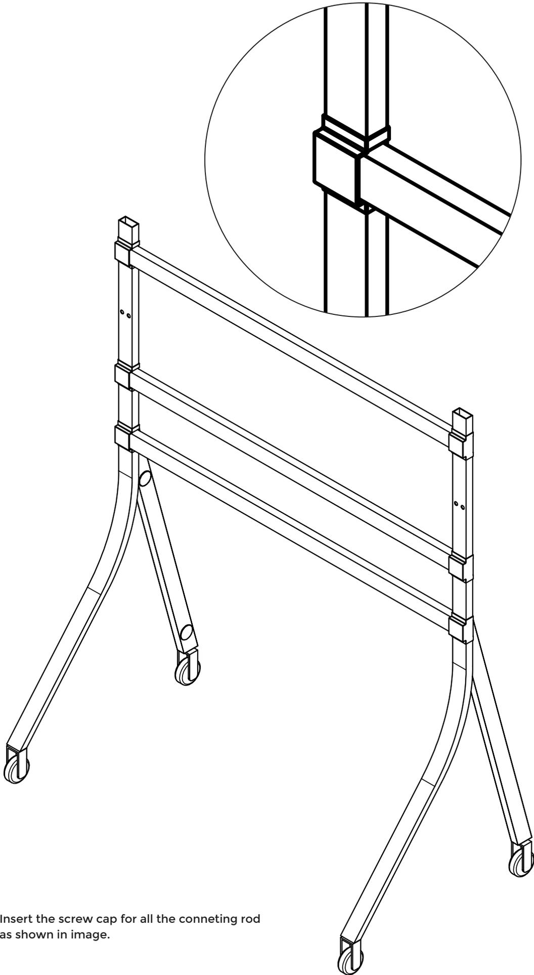
4. Insert the screw cap for all the connecting rod as shown in image.
