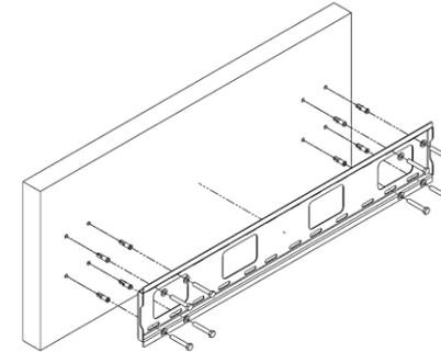
1. Place the wall unit on the wall and make marks on the wall.
