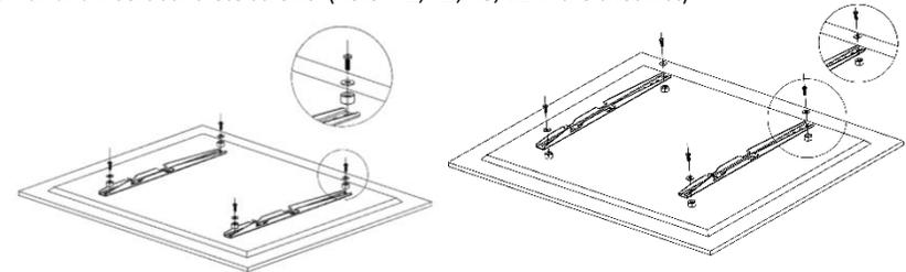
2. Place the interface bracket on the TV/ display and insert the washer and screw (Refer the checklist for the suitable screw and washer)
