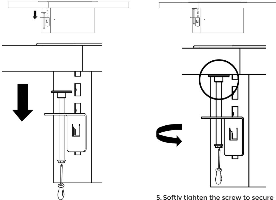
4. After positioning the cable manager into the table cut-out, insert the mounting clamp into the enclosure for securing the unit to the table surface (on both sides)
