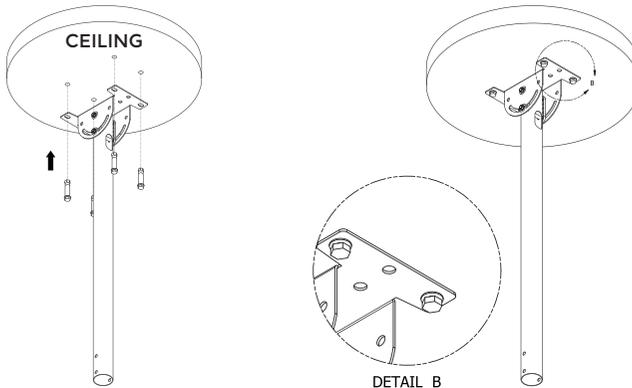
1. Place the ceiling mount on the ceiling mark on it and then drill, place the ceiling mount and insert the anchor bolt (Refer W-A in the checklist-kit)
