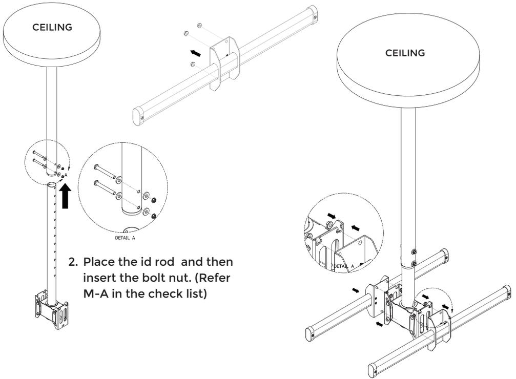
**3. Remove the nut from the horizontal bracket and place on the ceiling mount then insert the nut.**
