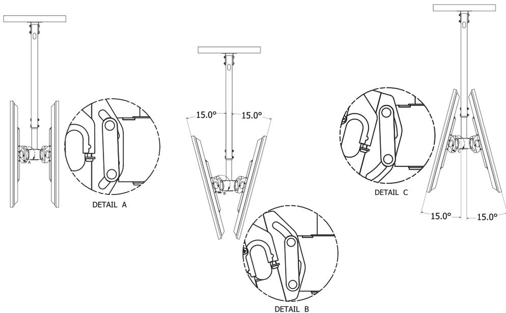
9. Slightly loosen the screw to adjust the angle
