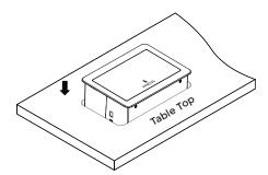
3. Then position the cable manager into the table cut-out
