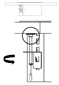
5. Softly tighten the screw to secure the enclosure towards the bottom side of the table (on both sides)
