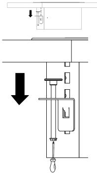
4. After positioning the cable manager into the table cut-out, insert the mounting clamp into the enclosure for securing the unit to the table surface (on both sides)
