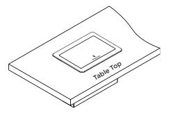
View after positioning the cable manager into the table
