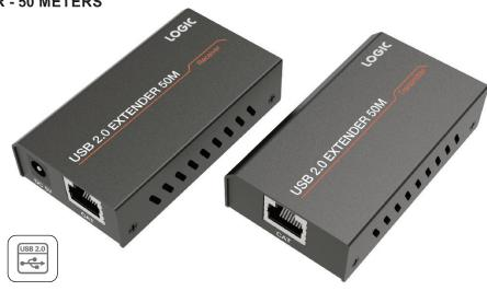
The USB2.0 extender can easily send the USB signals via CAT 5e/6 cables up to 50 meters /164 ft. at the transmission rate of 480 Mbps. Without any configuration or software driver. In a transmitter, the USB-B port has connected to a PC. In the receiver, you can connect a device with a USB port at the two USB ports such as a U disk or printer.
