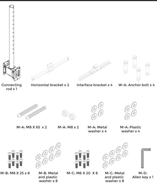
**IMPORTANT :** Ensure that you have received all parts according to the checklist prior to installation.
