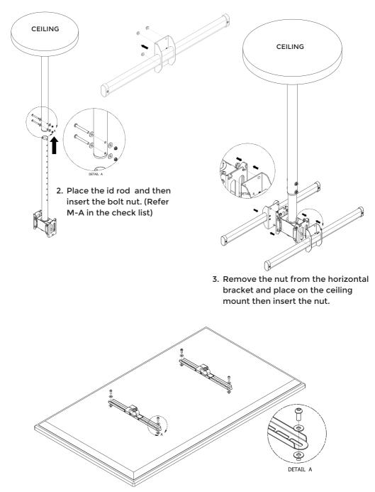
4. Place the interface bracket on the TV/ display and insert the washer and screw (Refer the checklist for the suitable screw and washer)
