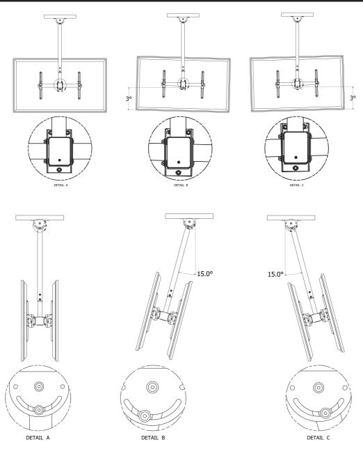
10. Slightly loosen the screw to adjust the angle
