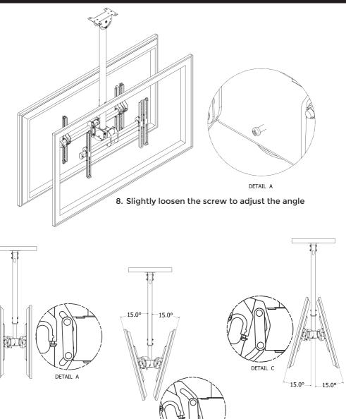
9. Slightly loosen the screw to adjust the angle
