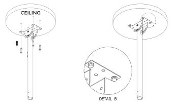
1. Place the ceiling mount on the ceiling mark on it and than drill, place the ceiling mount and insert the anchor bolt (Refer W-A in the checklist-kit)
