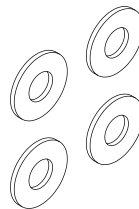
M-E: M8 washer x 8 (Metal washer x 4, plastic washer x 4)
