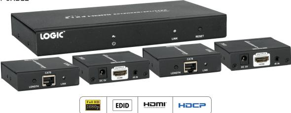
This HDMI extender splitter works with 4 HDMI CAT6 extender receivers to split and extend 1 HDMI source to 4 HDMI displays over single CAT6/6a/7 cable up to 40 m/131 ft.
