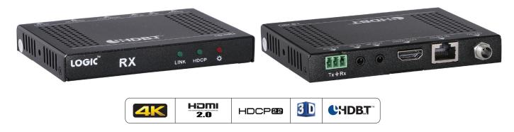
LG-HRx is a mini-size HDBaseT Receiver designed with HDBaseT technology to transmit high-resolution 1080p/4k signal from HDBaseT Transmitter to the LG-HRx via a CAT5e/CAT6a cable at a distance up to 70/40 m. Moreover, LG-HRx support CEC, bi-directional RS232&IR control, and unidirectional PoH function.
