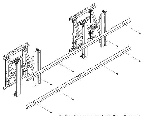
Fix the whole connecting bar to the wall mount bracket as show in image. Fasteners for fixing the bar is given in wall mount at connecting point
