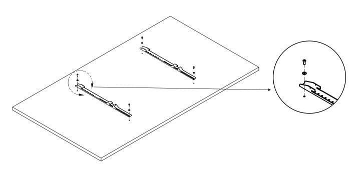
4. Place the interface bracket on the TV/ display and insert the washer and screw. (Refer the checklist for the suitable screw and washer)
