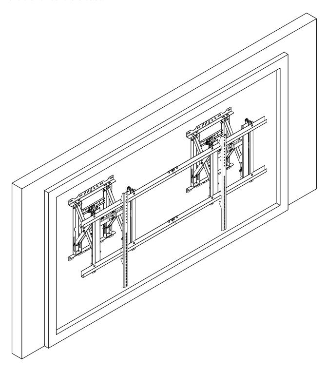
NOTE - Display cannot be unlocked at one push in middle. Since the display size is large.
