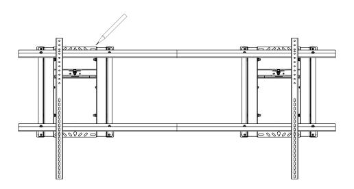
2. Place the unit on the wall and make marks on the wall.
