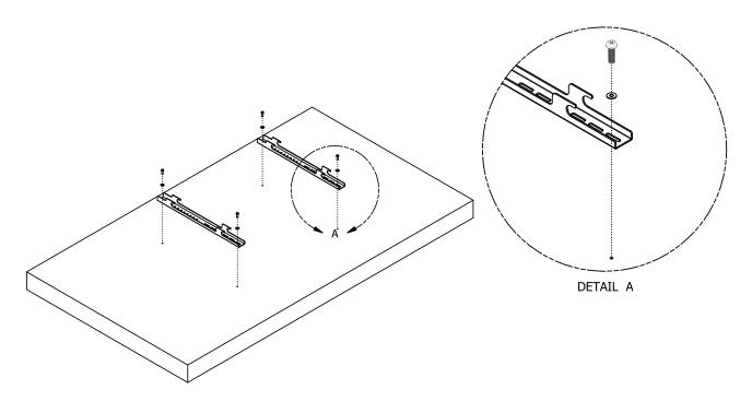
6. Place the interface bracket on the TV/ display and insert washer and screw (Refer the checklist for the suitable screw (M-C, M-E, M-G) and washer ( M-D, M-F, M-H) for the display/TV)
