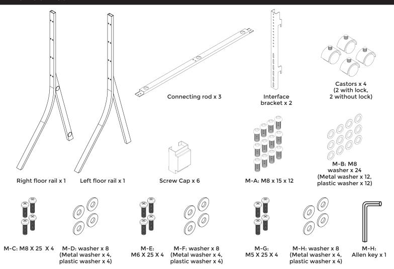
IMPORTANT: Prior to installation, ensure that you have received all the parts as per the checklist
