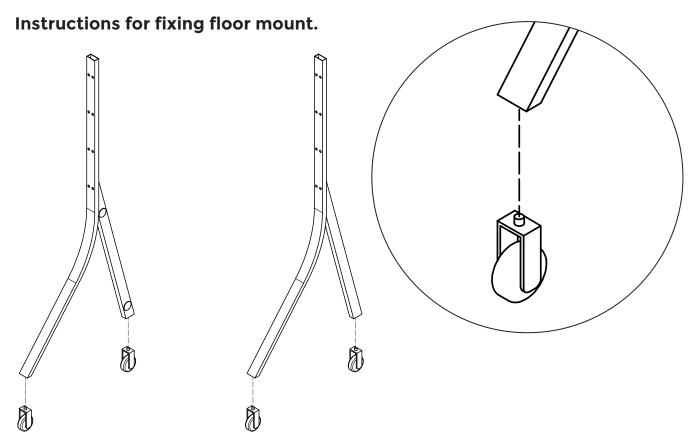
1. Place the castors to bottom side of the base left and right rail and tighten the castors
