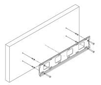
1. Place the wall unit on the wall and make marks on the wall. Note: While marking make sure the mount is placed in a straight line using the surface leveler Drill the wall and insert the concrete anchor in the holes & place the mount on the wall and insert concrete screws. (Refer A1, A2, A3, B1 in the checklist)
