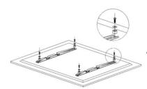
2. Place the interface bracket on the TV/ display and insert the washer and screw (Refer the checklist for the suitable screw and washer)
