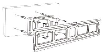
1. Place the wall unit on the wall and make marks on the wall. Note: While marking make sure the mount is placed in a straight line using the surface leveler Drill the wall and insert the concrete anchor in the holes & place the mount on the wall and insert concrete screws. (Refer A1, A2, A3, B1 in the checklist)
