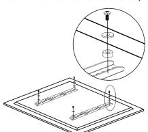
2. Place the interface bracket on the TV/ display and insert the washer and screw (Refer the checklist for the suitable screw and washer)
