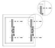
2. Place the interface bracket on the TV/ display and insert the washer and screw (Refer the checklist for the suitable screw and washer)
